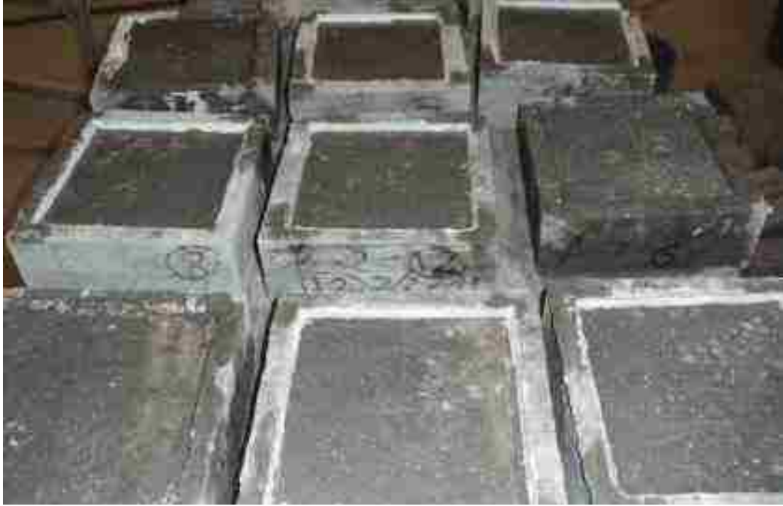
Figure 21 Surface scaling specimens during testing.
