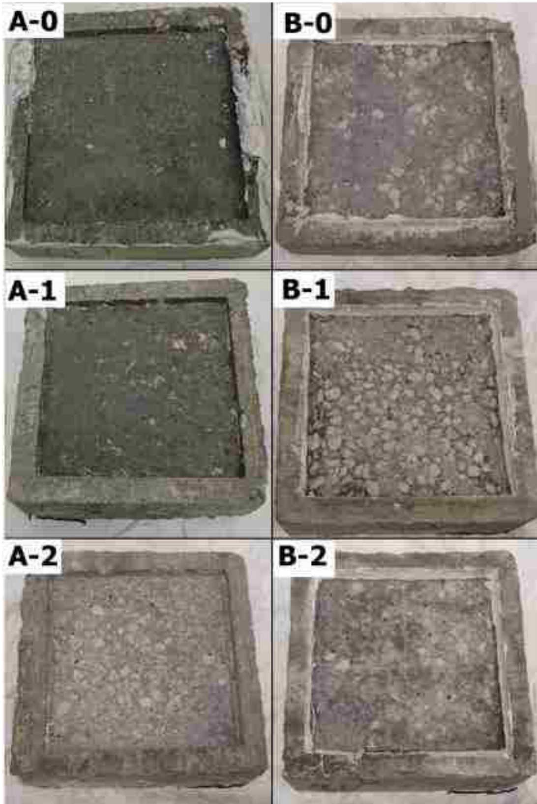
Figure 23 Scaling on the surface of the specimens after 60 cycles of exposure.
