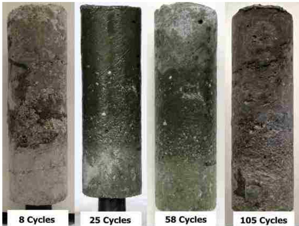
Figure 35 Damage in A-1 specimen at different ages of exposure.
