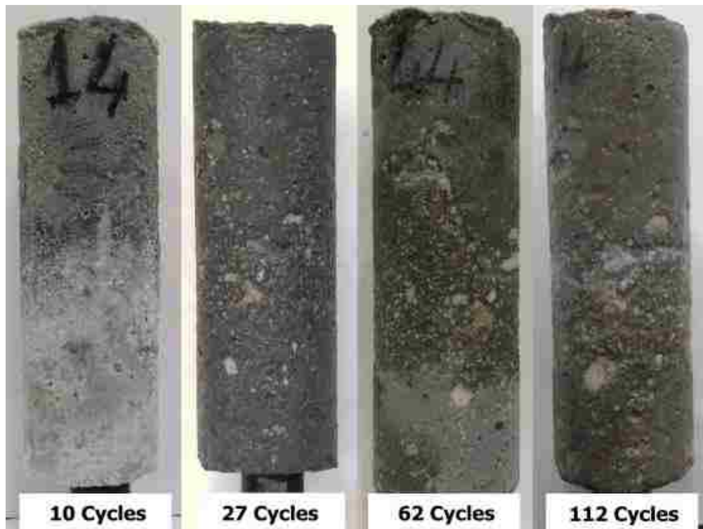
Figure 37 Damage in B-0 specimen at different ages of exposure.
