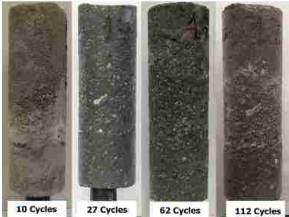
Figure 38 Damage in B-1 specimen at different ages of exposure.
